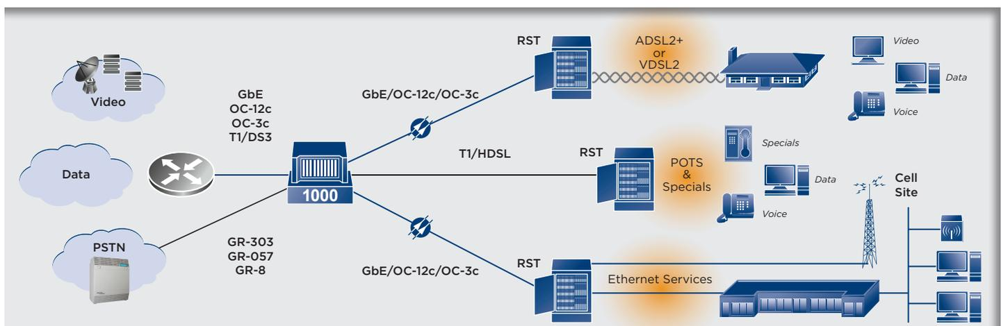
Figure 1. An optical transport uplink from the Tellabs 1000 MSAP leads to the core network to support multiple types of services.
