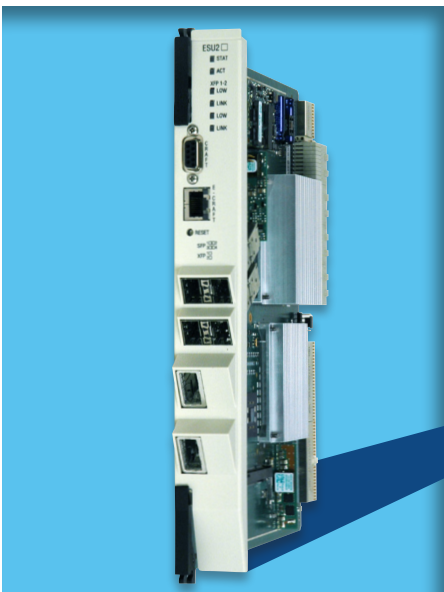
Tellabs® ESU2 Module 200G Full-Duplex Switch Fabric (Tellabs® 1150 and Tellabs® 1150E)
