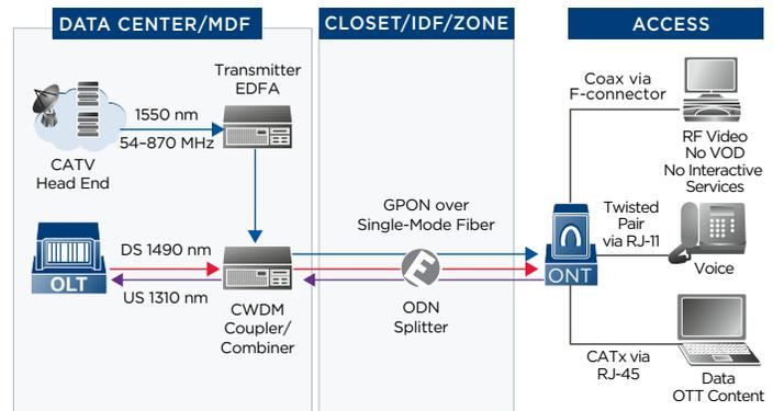
Figure 5: RF video over Optical LAN architecture
