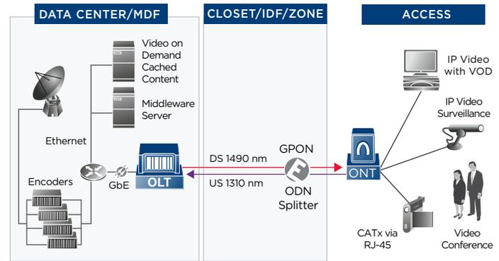
Figure 4: IP video over Optical LAN architecture
