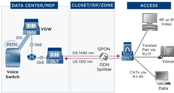
Figure 3: Analog (POTS) over Optical LAN architecture
